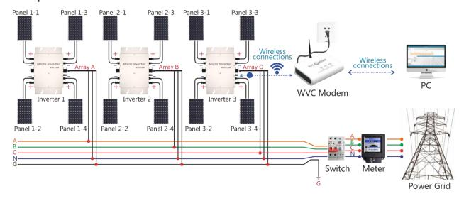
WVC-1200 (Wireless) Using IP65 waterproof streamline design, Can effectively prevent rainwater on the surface erosion, Built-in high-performance Maximum Power Point Tracking (MPPT) Function. Better able to track changes in the solar luminosity and control different output power, Effectively capture and collect sunlight. AC electric power transmission using the reverse transmission technology, Is one of our patented technology, The inverter output power can provide load priority use,
